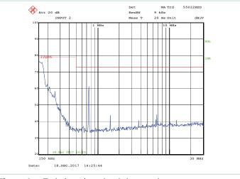
**Figure 1** — Typical conducted emissions, peak scan, with BCM4414VG0F4440T02 VIA, 400V<sub>AG</sub>, 90% load, no external components
