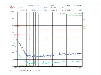
**Figure 2** — Typical conducted emissions, peak and average scan, with BCM4414VG0F4440T02 VIA, 400V<sub>AC</sub>, 90% load, with external components as shown in typical application on page 3
