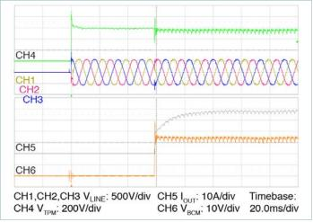
**Figure 5** — Start up from  $V_{IN}$
