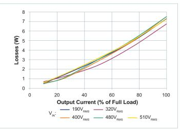
Figure 4 —  $V_{IN}$  to  $V_{OUT}$  power dissipation vs.  $V_{IN}$  (line to line) and  $I_{OUT}$ ,  $T_{CASE} = 25^{\circ}C$
