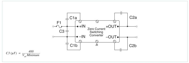
Figure 1 — Basic module operation requires fusing, grounding, bypassing capacitors.\* See <u>Design Guide & Applications Manual</u>.
